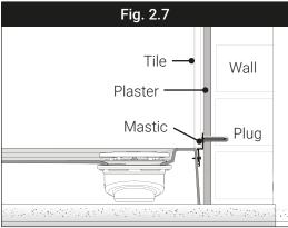
The waste cover and strainer can be removed to give clear easy access for rodding and to clear any accumulation of hair or other waste material.
